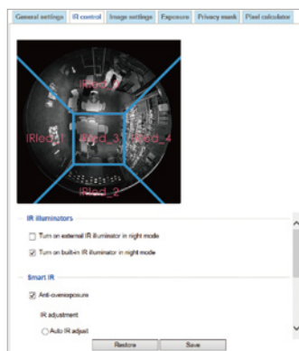
Independent IR control for regional illumination
